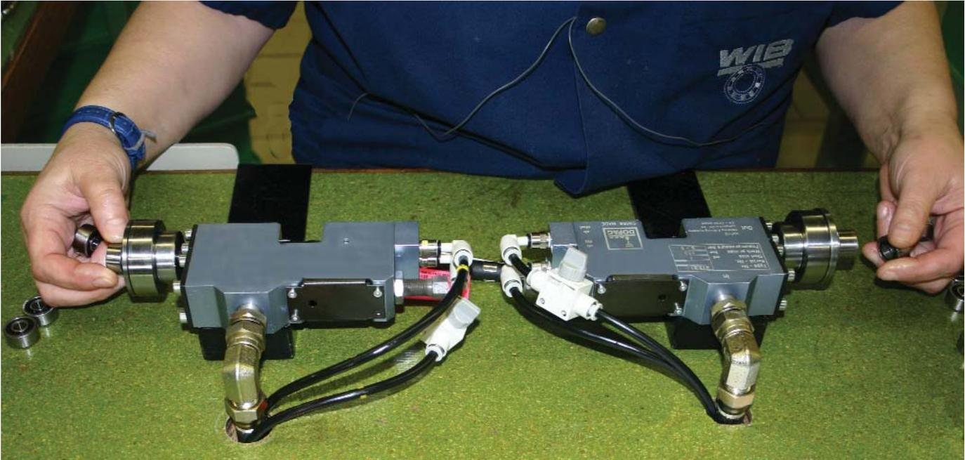
The operator offers up bearings to the twin DOPAG cartridge type metering valve
