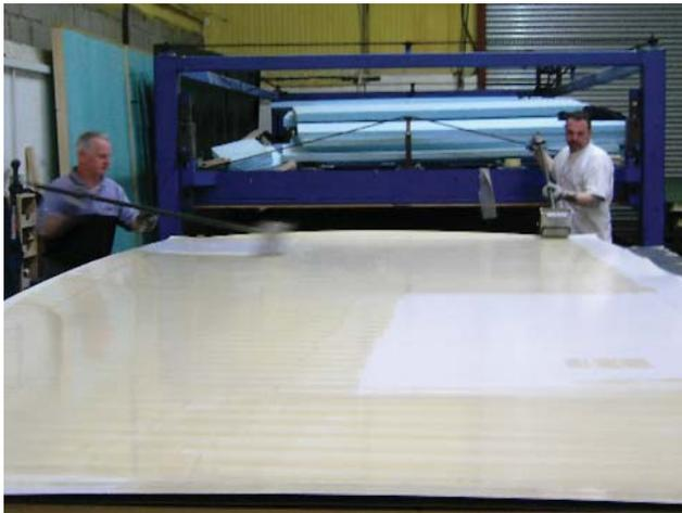
Laying the polyurethane onto a panel
