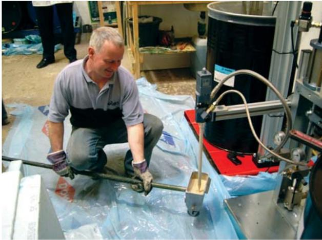
Filling the roller coater with mixed polyurethane
