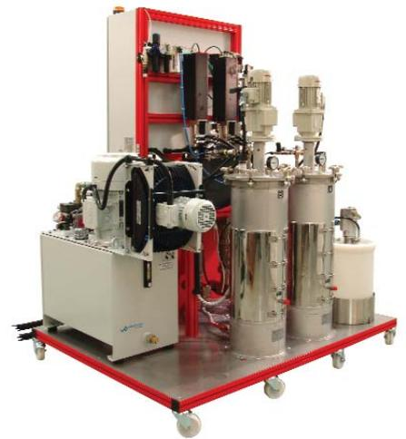
The pumps are fed with material from on-board pressure feed containers which are mounted onto a portable chassis, along with the hydraulic power pack.
