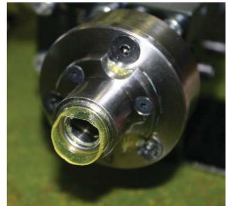
An end view of an applicator, clearly showing a metered shot of grease that would normally be injected into a bearing
