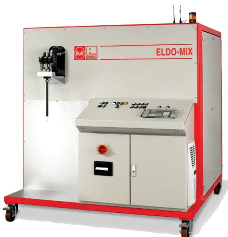
What follows is a brief insight into the first production stage where a vacuum supported infusion of a two component resin into fibre matting takes place.
