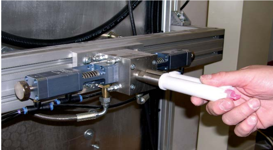
Filling the twin cartridge with the two component thixotropic silicone
