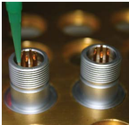
Dispensing mixed resin into a connector
