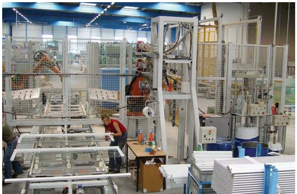
DOPAG P200 and P80 pumps (right) feed the DOPAG ELDO-MIX system (centre)
