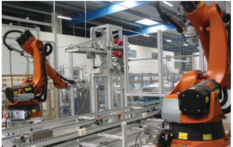
DOPAG ELDO-MIX system (centre) feeding a robot mounted dispensing valve (left)
