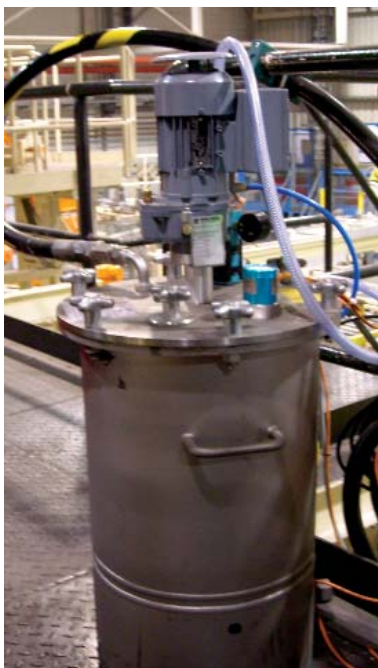
The adhesive is fed to the metering valves by a pressure feed container
