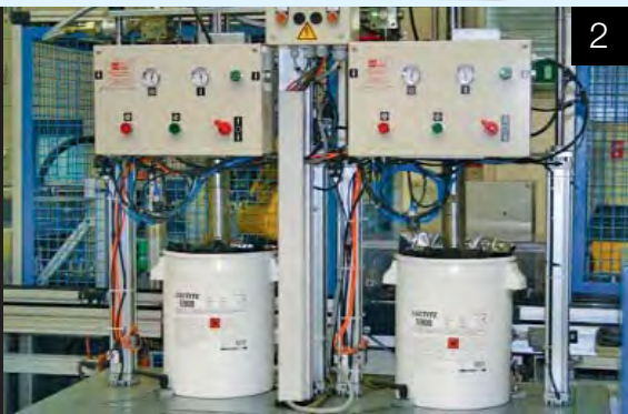
Twin DOPAG P30 drum pumps fitted with an automatic changeover system feed adhesive to the dispensing point
