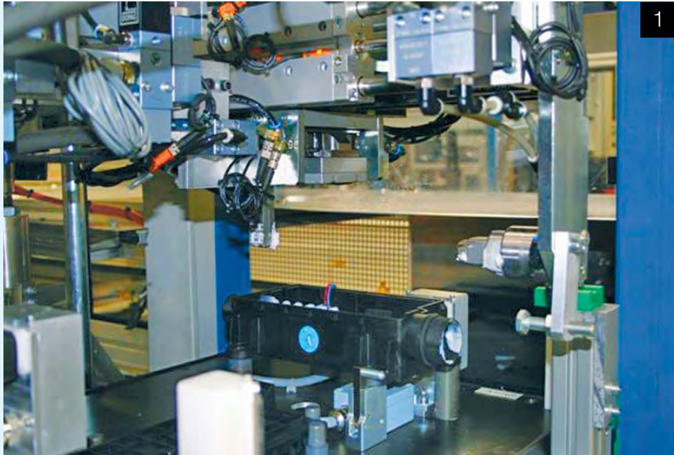
A chamber metering valve (top left) meters grease via a special fixture onto the brake unit mechanism
