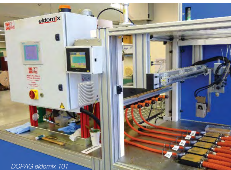
Proportioned and mixed polyurethane is metered into the electronic enclosure
