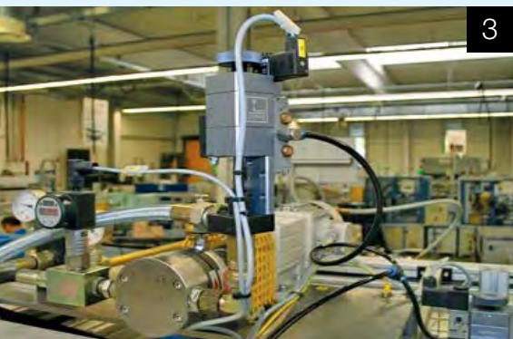
An in-line flowmeter checks the flow rate of the adhesive
