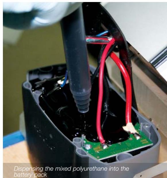
Dispensing the mixed polyurethane into the battery pack
