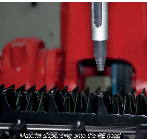
6-axis robot with a dispensing unit
