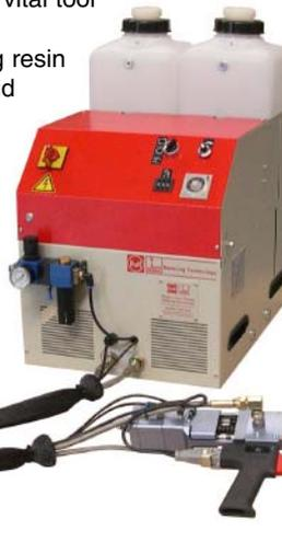
Following a successful demonstration at Hartlebury, Renault decided that the DOPAG ELDO-MIX 001 was the ideal machine to meter, mix and dispense the "parts-in-minutes" polyurethane resins supplied by material manufacturer, Huntsman.
