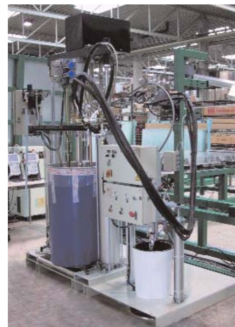
*Squeezing the silicone joint during assembly*
