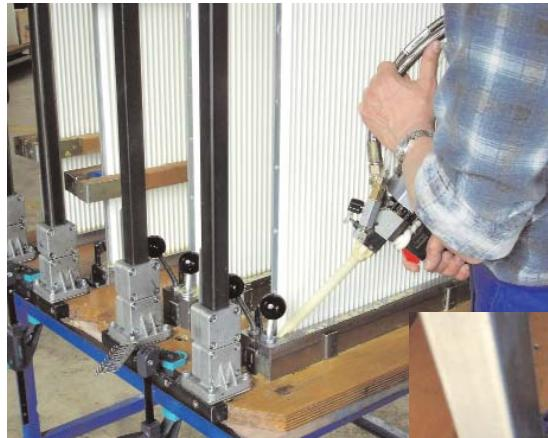
Mixed resin being dispensed into the fixture
