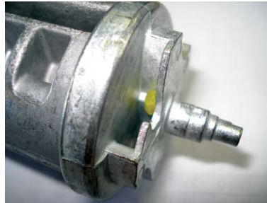
A seatbelt retractor spool showing the metered grease deposit
