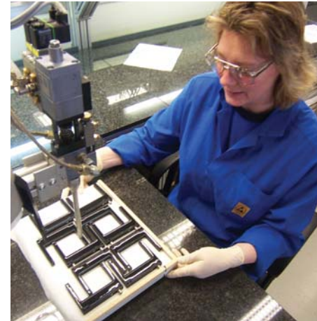
Sensor components are encapsulated with two component polyurethane using DOPAG ELDO-MIX 602 systems
