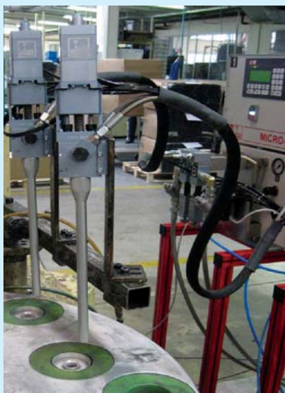
The DOPAG MICRO-MIX S dispensing stations
