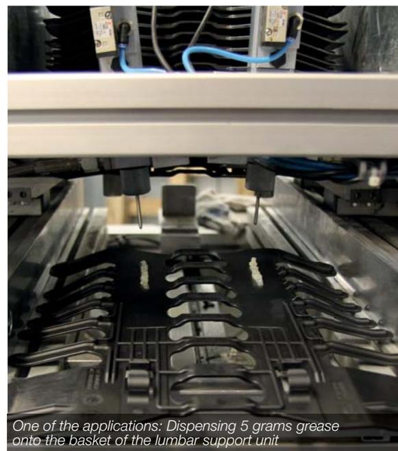
One of the applications: Dispensing 5 grams grease onto the basket of the lumbar support unit
