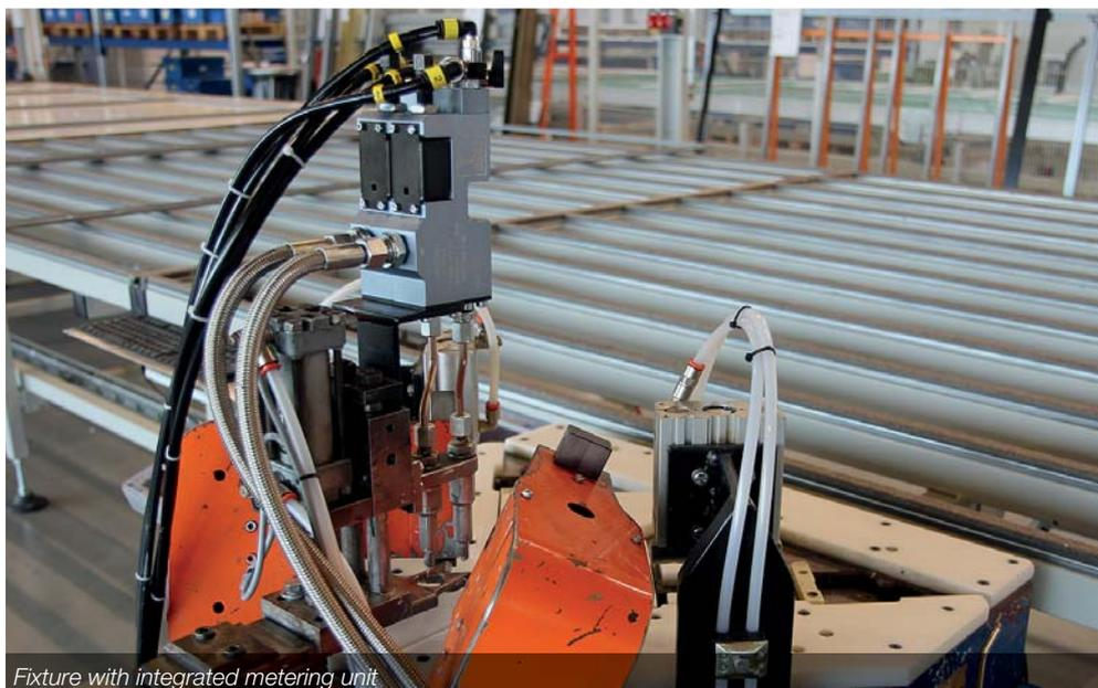
Fixture with integrated metering unit
