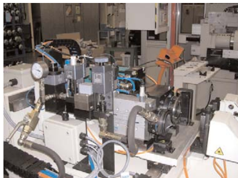
Electronic flowmeter grease metering module
